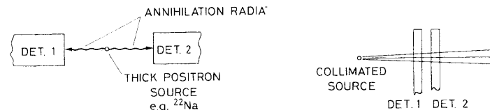
Fig. 15.10. Set-up for adjusting the coincidence between two detectors. For gamma ray detectors, the two photons from positron annihilation provide a useful source of coincident events. For charged particle detectors, a beam of electrons or other particles may be used provided the particle energy is high enough (and the counters thin enough) for the particles to pass through at least the first counter
